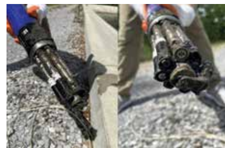
Figure 2. Multiparameter sondes with central wiper blade.
