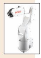
the company says. The robots feature ultraslim arms, an optional bottom-side cable connection and can be mounted on the floor, ceiling or wall.
