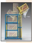
plant floor. The dumper allows boxes and other containers to be loaded at floor level, sealed against a discharge hood, elevated and tipped, mating the hood outlet
