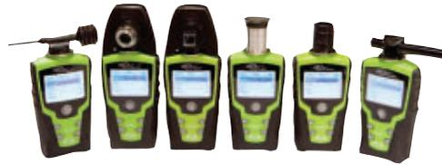
The i-Lab performs measurement and analysis of liquids and solids in the visible light range of 400-700 nanometers, according to MicroOptix Technologies.
