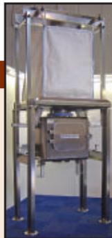
tions are interlocked to IP 67 for better dust/ingress protection, depending on the application and cleaning regime. A dust cabinet offers containment during discharge.
