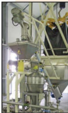
A flexible screw conveyor from Spiroflow Systems that moves dry bulk solids and ingredients features a direct electric motor-driven spiral screw. It is designed for speed, low maintenance and gentle handling. The conveying systems can be configured to operate in any direction and elevation
