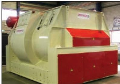
liquids can be oil-, water- or acid-based. The machine mixes quickly, making it possible to realize energy savings of 30% to 40%, according to the company.
