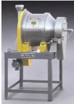
Co. blends batches up to 5 cubic feet, in parts as small as one per million, with uniformity in less than three minutes, according to the company. The stainless steel, sanitary unit features a stationary inlet and outlet for in-line operation and a rotating drum with proprietary mixing flights that tumble, turn and fold material gently.
