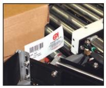
of the carton, according to company literature. The system can be integrated with most cartoner lines. A printer can be added to the system to print barcode, date or other production data.
