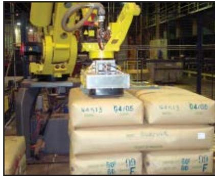
This system palletizes (or depalletizes) 100-lb. jumbo bags from two production lines simultaneously.
