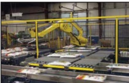
A robotic palletizer uses high-speed, full-layer forming techniques to arrange 20-50-lb. bags into full-layer patterns. The infeeds automatically change over via a touch screen.
