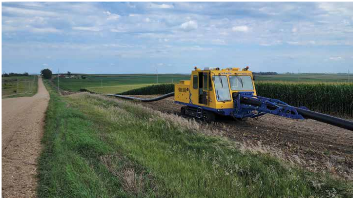
The Vietz Paywelder VFT 500 operator heat-fuses pipe sections together and controls the vehicle, speeding up the process. Photo courtesy of Douglas Westerman/ORWS.
