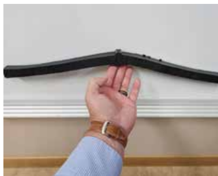
Douglas Westerman, general manager of ORWS, holds a cut section of an HDPE pipe joint used to perform a bend test proving that the heat-fused pipe sections will not pull apart. Photo courtesy of Douglas Westerman/ORWS.
