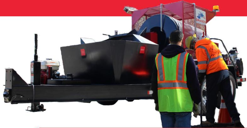
When using our **Mixer**, you can heat **650 lbs** of material to **350°F** in less than **10 minutes**. **No runs to the asphalt plant, no material costs & no waste.** The **Mixer** can also **recycle chunks of old raw road material.**
