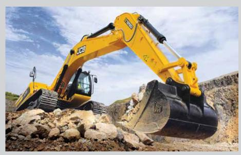
JCB's Tier 4 solution does not require a diesel particulate filter or exhaust aftertreatment, helping to make its excavators more fuel efficient and economical. For example, the JS200 has seen fuel consumption drop from around 6.0 gal. in 2010 to around 4.2 gal. currently, thanks to improvements in engine and hydraulic technology. Powered by a six-cylinder, Tier 4 Interim, 7.8-liter Isuzu engine, the JS360 achieves fuel savings of up to 8% compared with the Tier 3 version of the machine.
