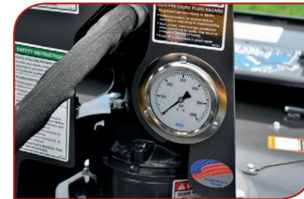
Standard pressure gauge indicator, easily visible to the operator helps prevent excessive stalling and overheating.
