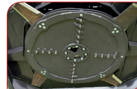
Optional 18 tooth carbide stump grinding kit increases mulching performance and takes the stump down to ground level. This option is highly recommended.
