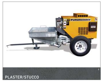
The Tommy Gun's 3-1/2" cylinder is ideal for high pressure, long distance plastering. Even the coarsest and most troublesome mixes will flow in a smooth easy-to-control stream, no matter how difficult the conditions. This mechanical piston ball valve pump also features a 2" outlet and 4-speed variable drive.
