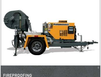
For high volume fireproofing, rely on the Tommy Gun with its large 3-3/4" cylinder, long 8" stroke and 3" outlet to deliver up to 60 bags an hour. This mechanical piston ball valve pump also offers 4-speed variable drive and an adjustable two-position stroke for the smoothest pumping.
