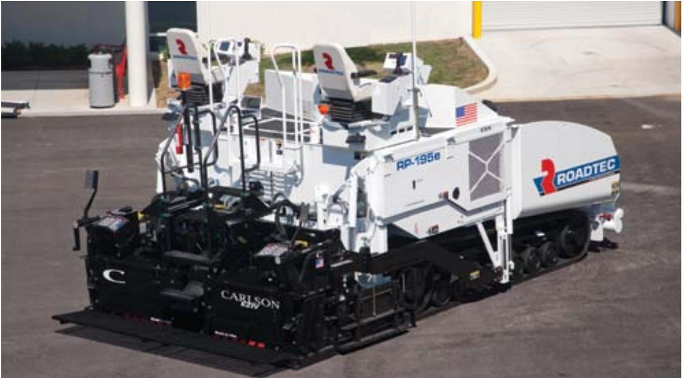
The RP-195e is a powerful, heavy-duty rubber-track paver for highway work offering operator comfort and safety with 360° visibility, fingertip controls, fully adjustable seats, low noise levels, and fume extraction systems. The exclusive Roadtec anti-segregation design gives consistent pavement quality. Dependable and tough.
