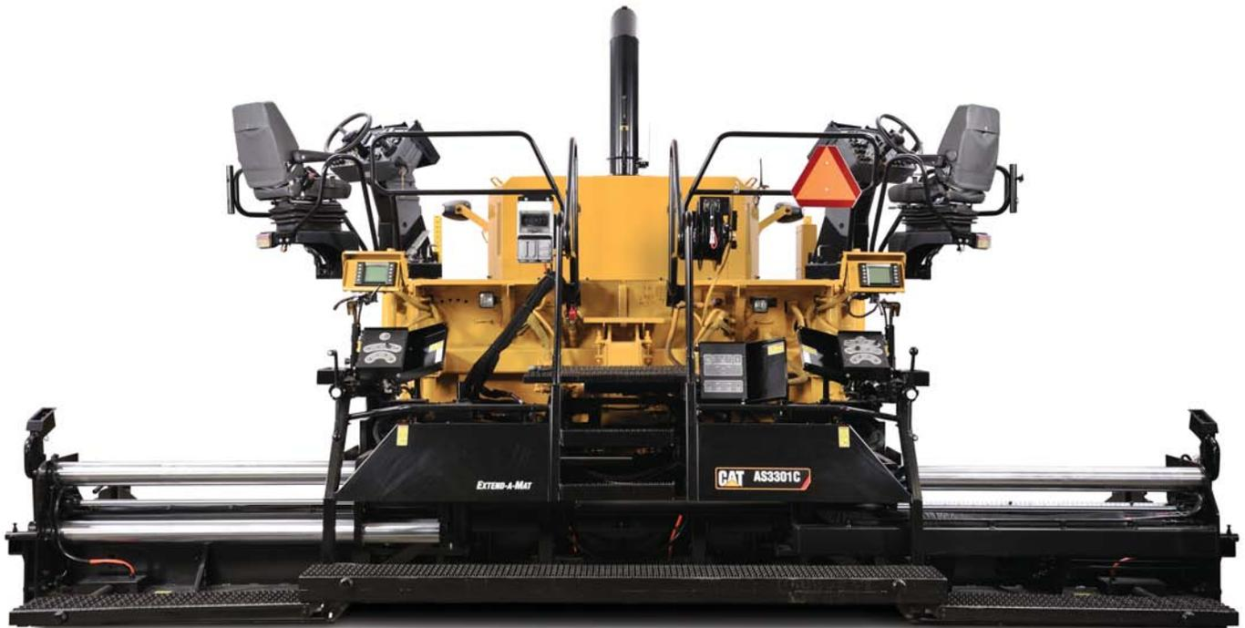
*Heavy-duty support tubes stabilize the extenders providing even material flow for high quality results on interstates, highways, airports and other high-production paving applications.*
